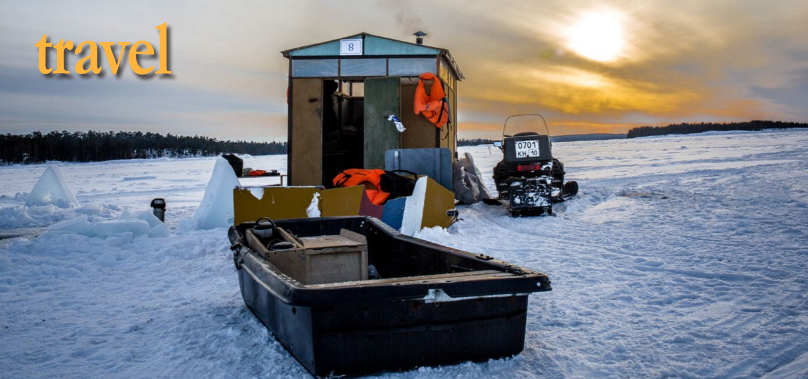
Ice diving ops on Lake Baikal use snowmobiles with trailers to transport divers, warming huts and equipment from site to site
