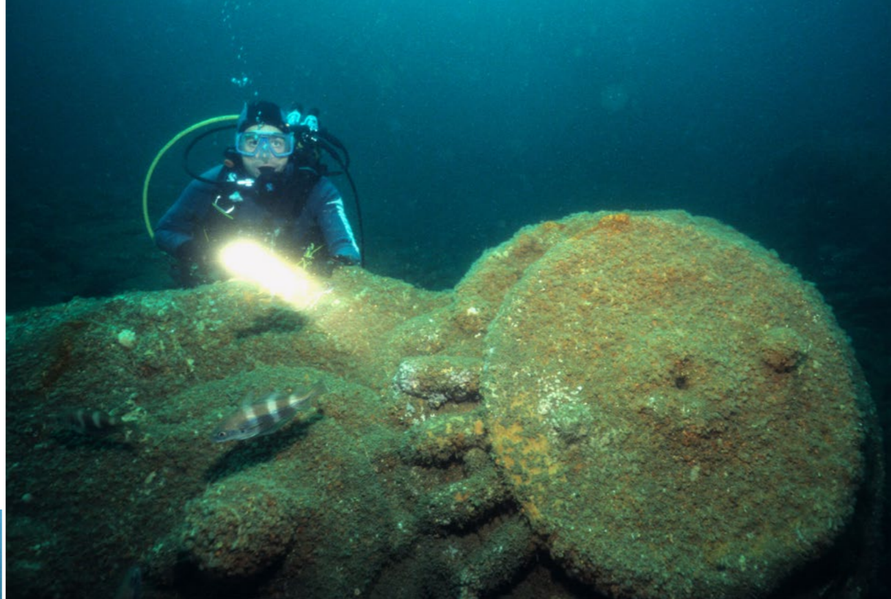
Top of the smaller cylinder of the engine, which is lying down on the starboard side (right); Top of the main cylinder of the triple expansion steam engine (below)
