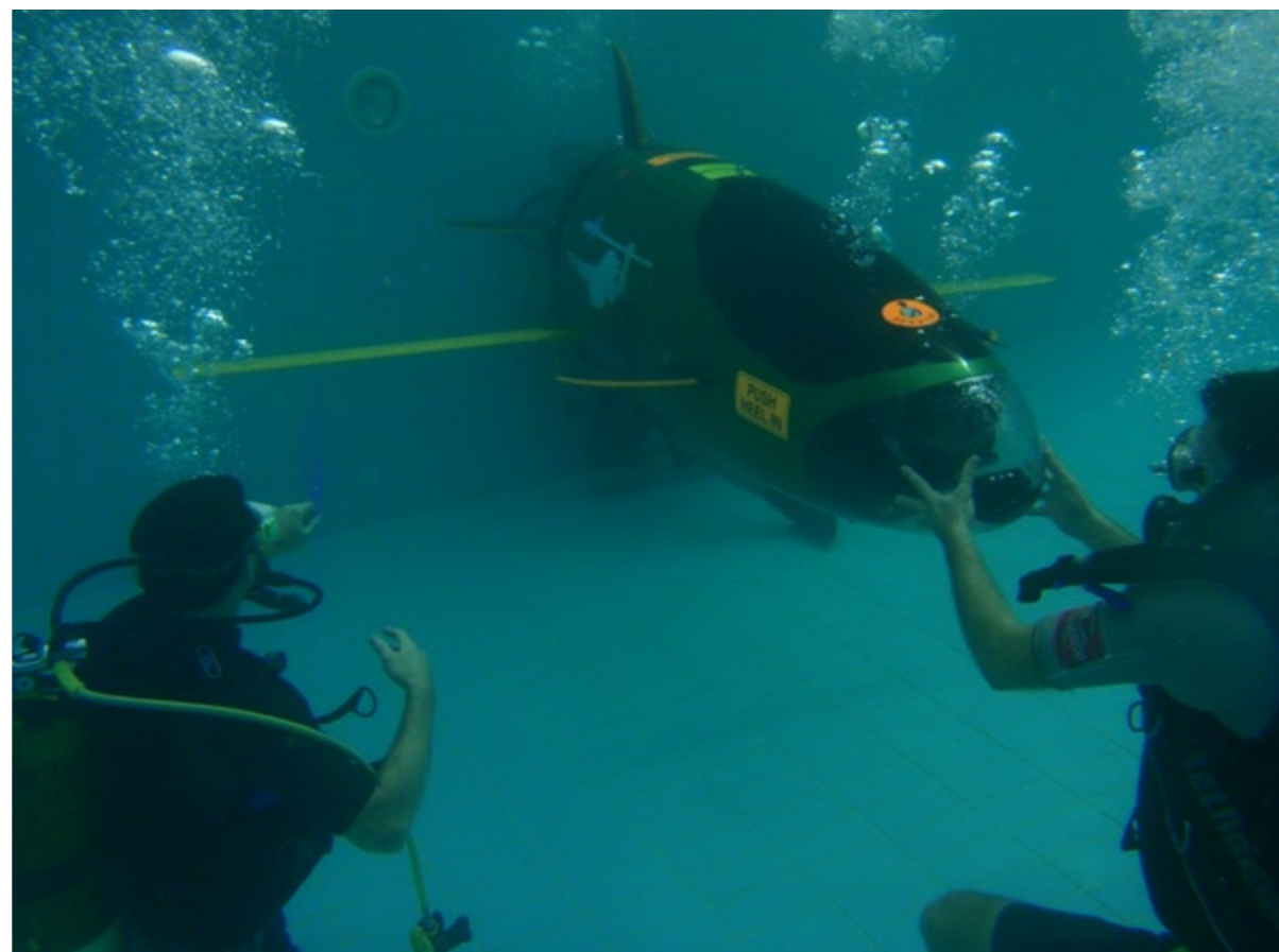
The Omer submarine team from the Université du Québec's École de technologie supérieure in Montreal, Canada, trim the buoyancy of Omer 6 as Lloyd pedals the submarine from one side of the pool to the other
