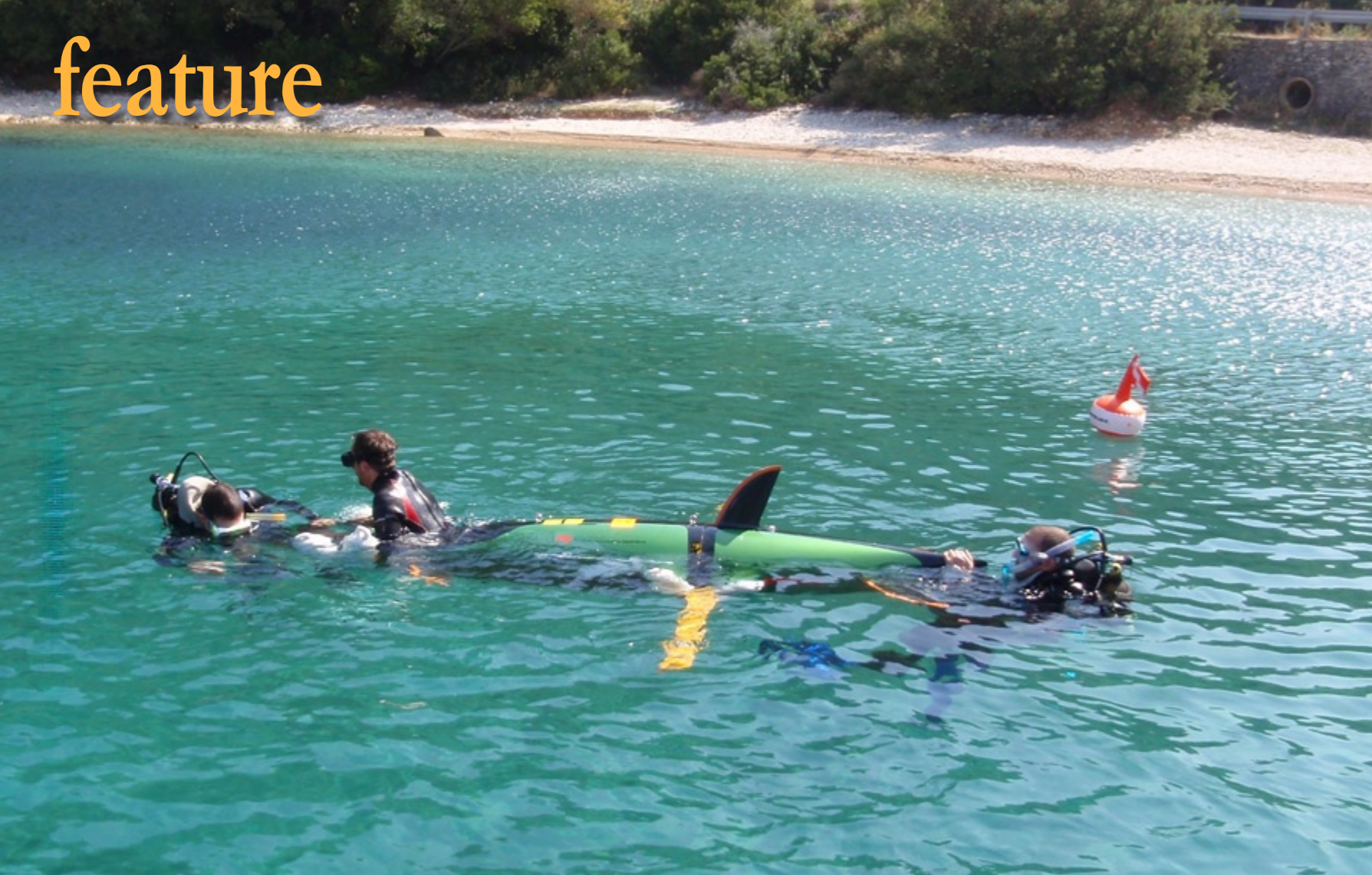
Lloyd Godson enters Omer 6—the human-powered submarine he used for the Life Amphibious expedition. Omer 6 is what's known as a "wet" submarine, meaning it's completely filled with water.
